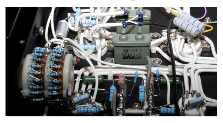
The I60 and M60 are entirely built using handselected, precisely matched components. Custommade military-spec paper-in-oil capacitors, tantalumfilm resistors are used in the signal path. Low noise gold plated ceramic tube sockets are used for every tube, and solid-core silver wiring is used throughout.
