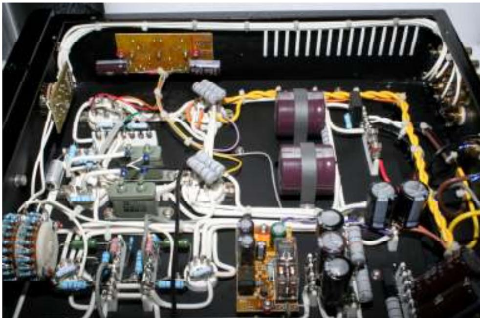
During construction, all components are hand-selected and precisely matched. The output transformers *and* power transformer are laboriously hand wound to precise specifications tailored to the circuit and tubes used.
