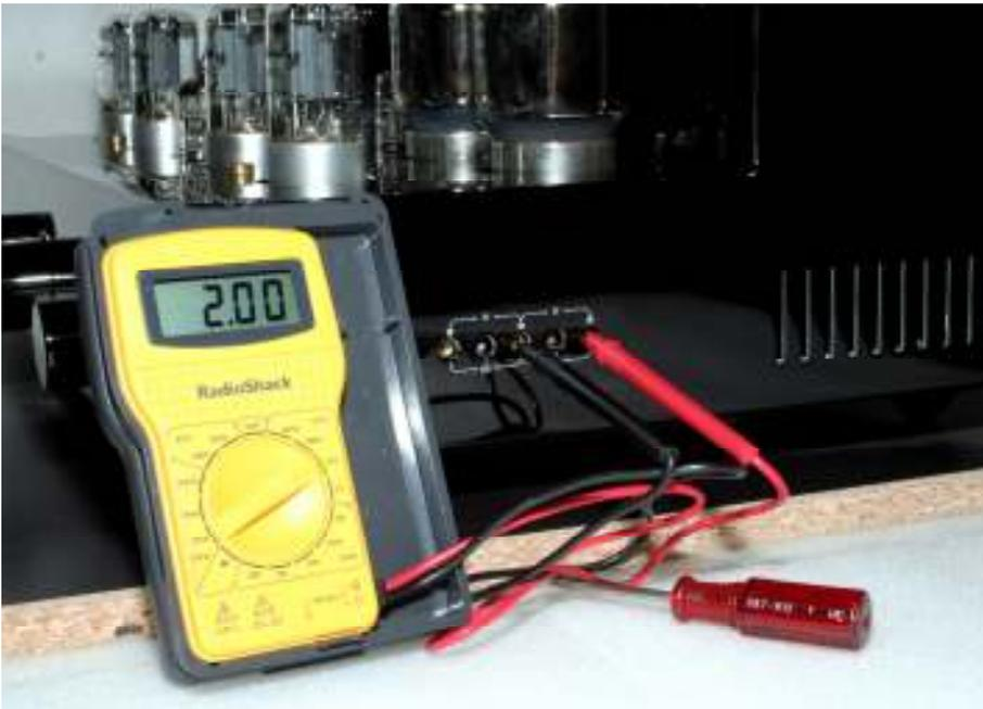
Poke the red probe of the multimeter into the hole labeled (+) and the black probe into the hole labeled (-).
