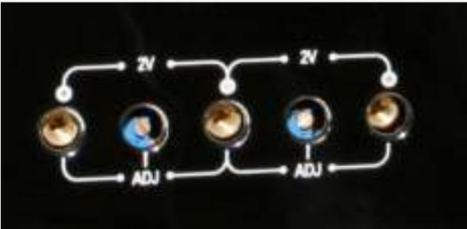
On each side of the I60, you will see a set of 5 little holes. Three of the holes are for the probe of a multimeter, and two that give you access to a little screw. Each set of holes is used to adjust the bias for the two output tubes of a single channel (left or right).
