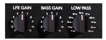
The knob in the middle marked BASS GAIN controls the volume of the built-in bass servo amplifier. Begin with this control at the 12 o'clock position (marked 6 on the scale). The knob on the right marked Low PASS controls how high in the frequency range the woofer will play. At the extreme low of
