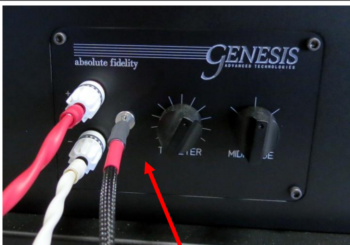
The Servo-Bass Interlink connects the crossover of the midrange/Tweeter to the input of the Servo-Bass Control Module.
