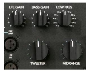
The knob on the upper middle marked "**Bass Gain**" controls the volume of the built-in bass servo amplifier. Begin with this control at position 7. The knob on the upper right marked "**Low Pass**" controls how high the woofer will play. At the extreme low of 71Hz, the woofer will play up to 71Hz, and then begin rolling off, or reducing its volume. The recommended beginning position for this control is 90Hz.
