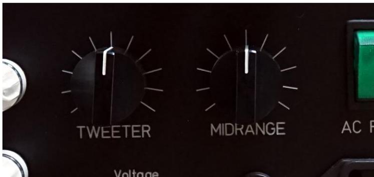
The lower left knob on the back plate marked "**Tweeter**" is a volume control for the front tweeter. Turning this control clockwise will increase the level of the front tweeter. Use this control if you need a bit more treble or to increase the apparent space of the soundstage. Start with this control at the 12 o'clock position. There is a +/- 1
