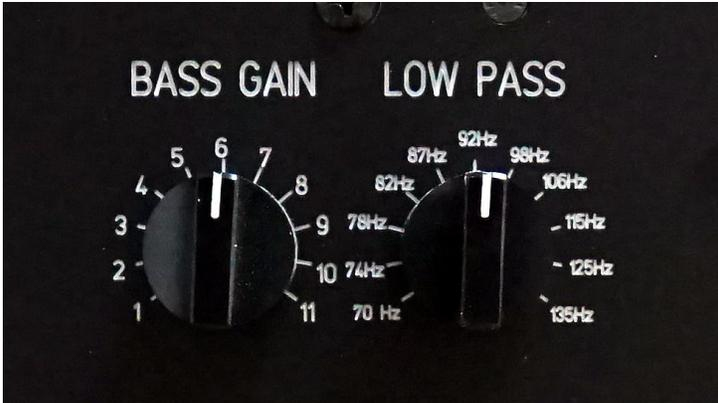
The knob on the middle of the lower row of knobs marked “**Bass Gain**” controls the volume of the built-in bass servo amplifier. Begin with this control at 6 (the 12 o’clock position). Adjusting the gain higher will make the loudspeaker sound “fuller” and more bass-heavy.
