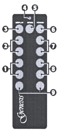
At this point, you can turn on the woofer amplifier ③. Using the remote control, turn on the subwoofer amplifier by pointing the remote control at the small remote enclosure. Adjust the phase ② to 40 with the button marked "phase" on the remote control. Next, adjust the low pass filter ③. Set this to 85 using the button marked "low pass". Next, adjust the volume to 30 to begin with. The volume will always flash to identify itself. Make sure the woofer works by playing some music.
