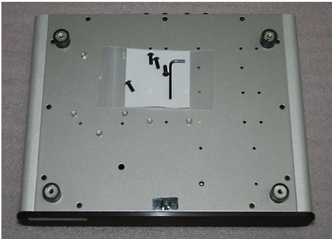
Place the amplifier chassis top down on a clean surface. Place the suspension frame on the shock absorbers so that the holes of the shock absorbers are aligned with the matching holes on the frame. The suspension frame “points” forwards so that the tip of the triangle faces to the front of the amplifier, and the round hole is in the front.
