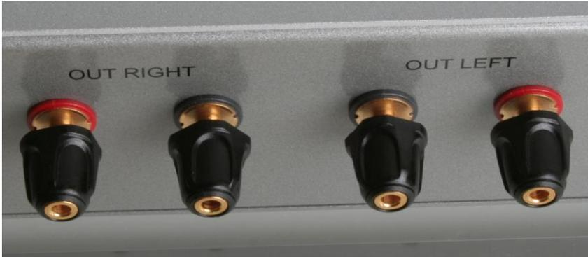
The binding posts are ETI CablePods™ for improved signal transfer, enhanced sonic performance, and a faster, more direct connection. The positive (signal) terminal is identified by the red ring on the base; and the negative (return) terminal is identified by the black ring on the base.
