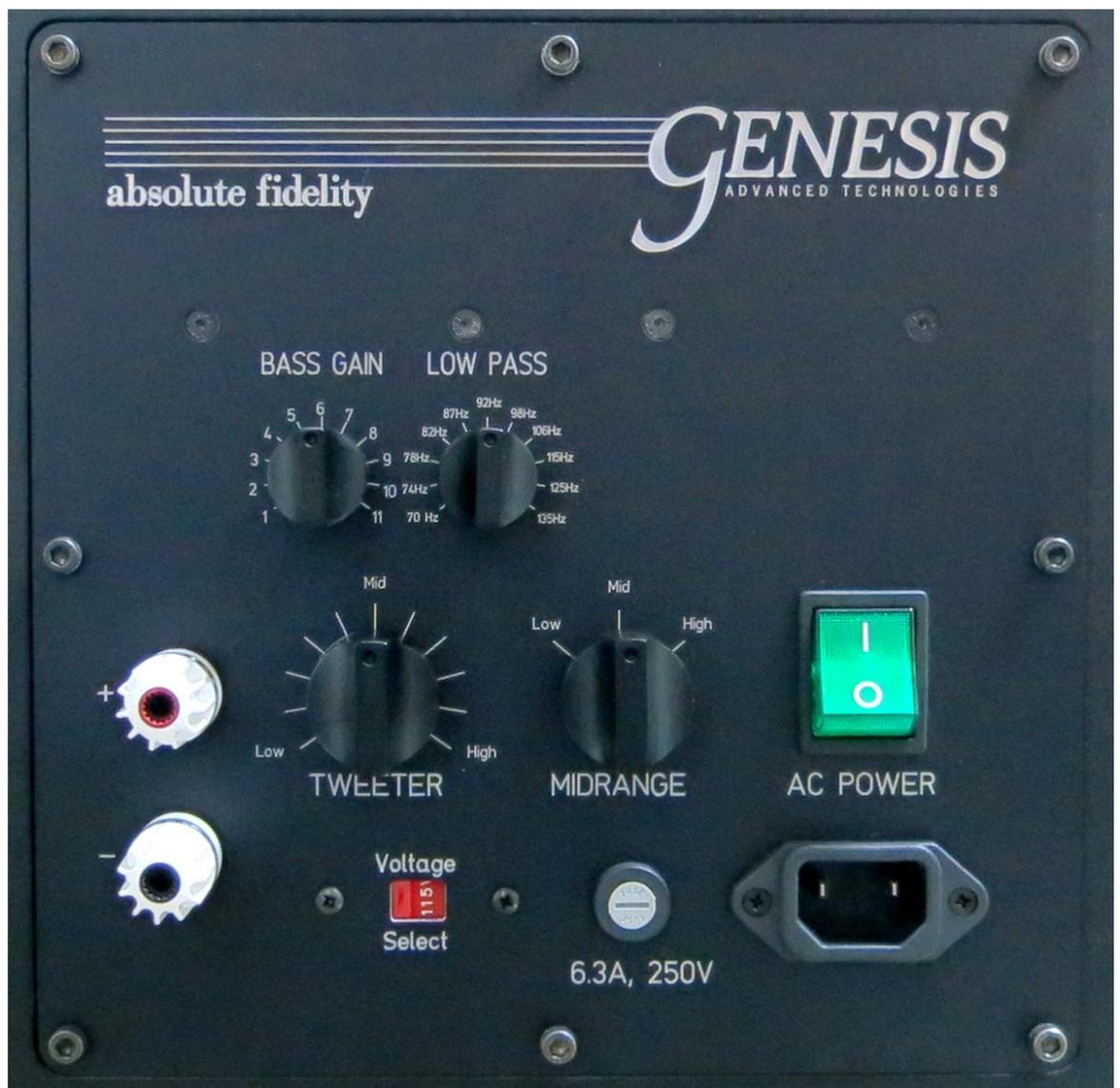
minimum-sized room, the bass gain should be set at 3 (the 9 o'clock position), and the low-pass at 92Hz (the 12 o'clock position).
