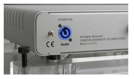
Locate the power toggle switch on the back next to the power umbilical inlet and **flick** it **upwards** to turn the amplifier ON.
