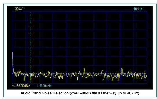
The electronics used for regulation have to be noiseless and fast. Generally noiseless is not a problem but fast is a great problem. Most commercial regulators are good for about 100 kHz. Most chokes are good for at least 1 MHz.
