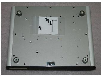
Place the amplifier chassis top down on a clean surface. Place the suspension frame on the shock absorbers so that the holes of the shock absorbers are aligned with the matching holes on the frame. The suspension frame "points" forwards so that the tip of the triangle faces to the front of the amplifier, and the round hole is in the front.
