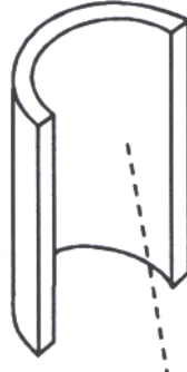
1/2 inch thick semicircular wood fiber tube to be affixed to the Genre enclosure.
