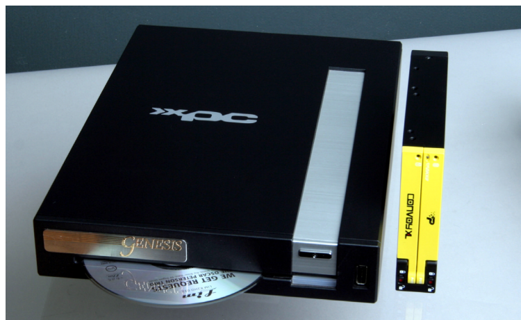
The Genesis Music Server is built around a Shuttle XPC and a 1 TB RAID2 drive
