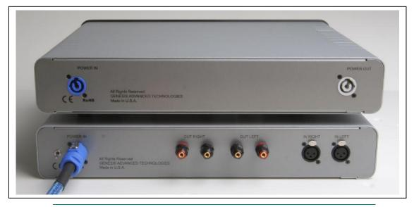
2) Turn off the amplifier using the toggle switch (if it is not already turned off) and unplug the blue Neutrik connector on the Power Umbilical from the back of the amplifier, and plug it into the blue Neutrik inlet on the back of the MDHR.
