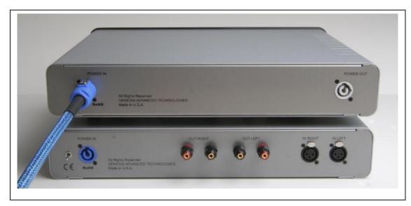
3) Plug the grey Neutrik connector on the short Power Umbilical supplied together with the MDHR into the grey Neutrik outlet on the back of the MDHR.
