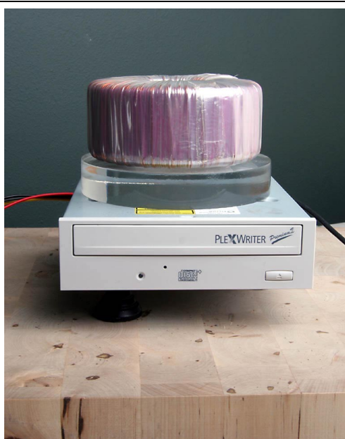
Plextor PlexWriter Premium-II on top of Ikea butcher's block; spikes are screwed into the block and point up to couple
